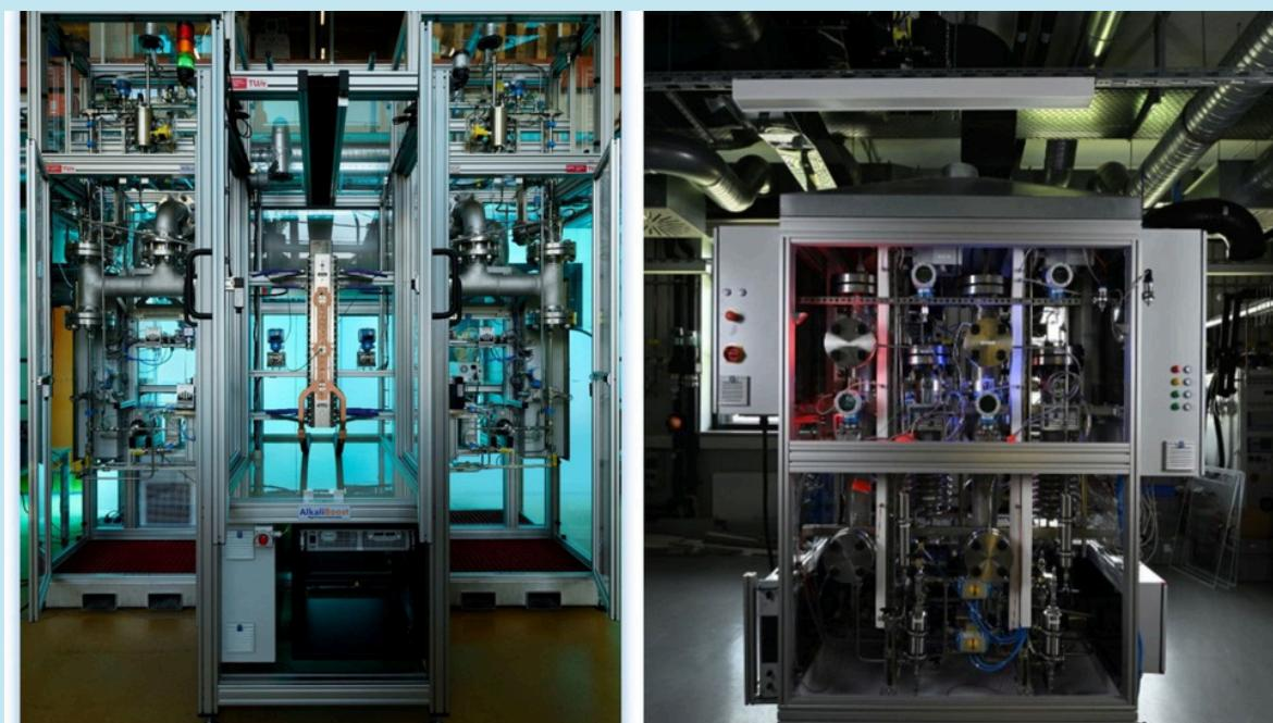
Facility used for electrochemical performance testing under pressurized conditions within the PEACE project (left: at TU/e, right: at DLR), Source: TU/e & DLR (CC-BY-NC-ND 3.0)
